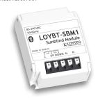
The LOYBT-SBM1 is a compact actuator for sunblinds in a Bluetooth Mesh ecosystem. It is based on a Bluetooth SIG qualified stack and integrates perfectly into the LOYBT product line and LOYTEC controllers with Bluetooth Mesh interface. The device is mains- powered and comes with 2 built-in relay contacts, which are suitable to switch currents of up to 6A at 250 V AC.
