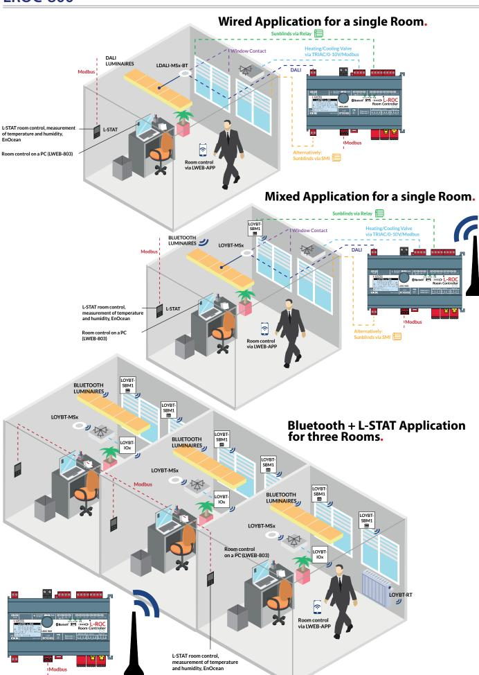
The LROC-800 Room Controller can control 3 room segments. Based on the various room segment types, larger buildings can be modeled in a hierarchical manner. Areas are built with an area manager by combining multiple room controllers. A floor manager manages multiple areas in one floor. Depending on the architecture, the building can be split up into areas and floors as needed.
