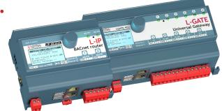
The L-IP Routers LIP-1ECTC, LIP-13-ECTC, LIP-3ECTC, LIP-33ECTC, and LIP-3333ECTC connect twisted pair channels (TP/FT-10 or TP/XF-1250) with the Ethernet/IP channel (IP-852) in LonMark Systems. L-IP routes CEA-709 packets through an IP based network such as a LAN (Ethernet), an Intranet, or even the Internet.
