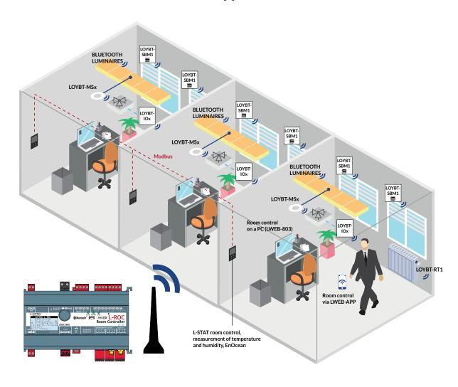
The LROC-800 Room Controller can control 3 room segments. Based on the various room segment types, larger buildings can be modeled in a hierarchical manner. Areas are built with an area manager by combining multiple room controllers. A floor manager manages multiple areas in one floor. Depending on the architec-
